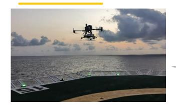
Drone 9kg CO2 + CH4 sensor Drone-mounted diode laser spectrometers Whole site or specific areas
